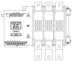
Solderless, screw-type terminal lugs are standard. Conductor sizes must be adequate to handle the maximum current to which they will be subjected; based on the 75°C column of tables, charts, etc. used to size conductors. The installation must comply fully with all applicable codes, standards and regulations.
